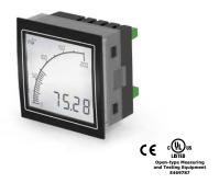
The APM Shunt Meter is for use in low-side DC current measurement applications where precise accuracy is required. It is able to measure to an accuracy of 0.1% of the signal or 0.5mV, whichever is greater.
