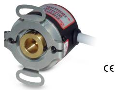
Miniature high precision encoder with a 10mm blind hollow shaft it has a 125Khz frequency response and can mount directly onto motor shafts. Quadrature output and Flexible mounting bracket.
