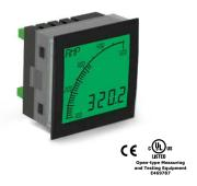
The APM Amp Meter provides effective measuring and monitoring of currents up to 5A directly, or up to 1,000A in conjunction with a current transformer.
